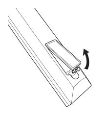
2. Load two batteries ("AAA" size, 1.5 V) matching the polarity.
